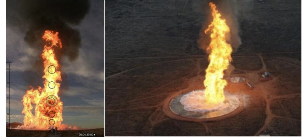
LNG Test 2 – 83m diameter spill and pool fire (US Department of Energy, 2012)
